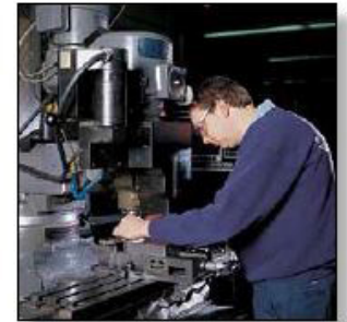
Machining a custom-engineered bending die in the Eagle tool room.
