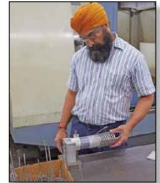
Adjustments being made to a heat exchanger part after coiling operation.
