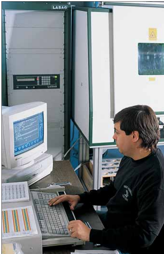
Computer controls laser welding equipment enabling extremely close-tolerance cutting, notching, etching and welding operations.
